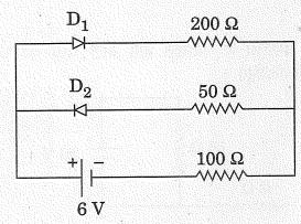
The circuit shown in the figure contains two diodes each with a forward resistance of 50  $\Omega$  and infinite backward resistance. Calculate the current in the 100  $\Omega$  resistance.
