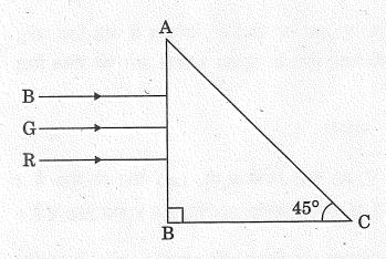
Three rays of light, red (R), green (G) and blue (B), are incident on the face AB of a right angled prism, as shown in the figure. The refractive indices of the material of the prism for red, green and blue are 1.39, 1.44 and 1.47 respectively. Which one of the three rays will emerge out of the prism? Give reason to support your answer.
