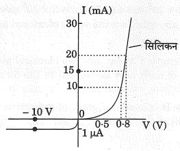
The V-I characteristic of a silicon diode is as shown in the figure. Calculate the resistance of the diode at (i) I=15 mA and (ii) V=-10 V.
