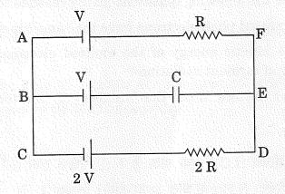
In the given circuit in the steady state, obtain the expressions for (a) the potential drop (b) the charge and (c) the energy stored in the capacitor, C.
