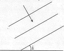
A plane wavefront propagating in a medium of refractive index ' $\mu_1$ ' is incident on a plane surface making the angle of incidence 'i' as shown in the figure. It enters into a medium of refractive index ' $\mu_2$ ' ( $\mu_2 > \mu_1$ ). Use Huygens' construction of secondary wavelets to trace the propagation of the refracted wavefront. Hence verify Snell's law of refraction.
