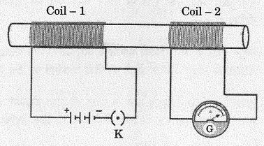
(i) Why does the galvanometer show deflection only when the key (K) is plugged in and not when a steady current starts flowing in the circuit?
