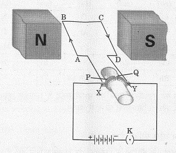
As shown in the figure, the current in the coil ABCD flows from A to B in the arm AB and C to D in the arm CD.
