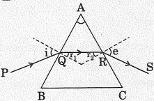
Figure shows a ray of light passing through a prism. If the refracted ray QR is parallel to the base BC, show that (i)  $r_1 = r_2 = A/2$ , (ii) angle of minimum deviation,  $D_m = 2i - A$ .
