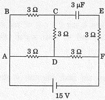
In the circuit shown in the figure, find the total resistance of the circuit and the current in the arm AD.
